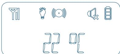
HI TEMP = Baby unit temperature alert > 30 °C
