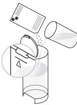
**3 Pour 1 Nespresso descaling liquid sachet into the water tank. Fill the water tank up to the 0.6 L line with portable water.**
