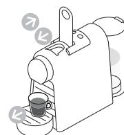
**5 Remove the cup.** Lift and close the lever to eject the capsule into the used capsule container.
