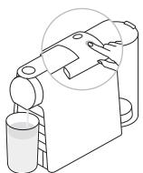
**7 Press the Lungo button and wait until the water tank is empty.**
