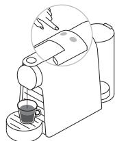
**4 Press the Espresso** (40 ml) or the Lungo (110 ml) button to start. Preparation will stop automatically. To stop the coffee flow or top up your coffee, press again.
