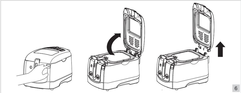
**CLEANING AND MAINTENANCE - Replacing the oil or liquid fat**
