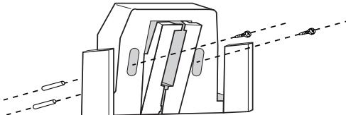
Figure 2 Mounting the charging holder to a wall
